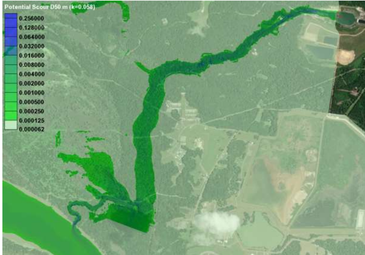
Figure 3. Results of critical erosion mean grain size (d50) calculations in Lily Bayou. Grain size diameters are in meters and 0.058 is used as k (equations 3 and 4). Contour Ranges are from green (smallest diameter) to blue (largest diameter) and are divided by associated grain size classification with the lightest green equivalent to very fine sand and the darkest blue corresponding to boulders. The raster layer of this file is “comited50_058.tif”.
